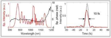
Left: Spectrum (red) after broadening in a 6 m SF-HCF fiber and phase (blue) after compression.
