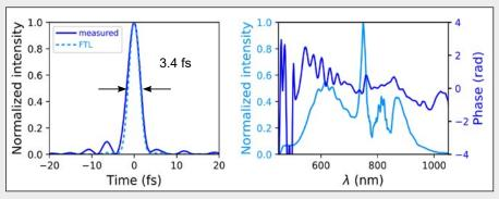
Left: Retrieved temporal profile and ideal Fourier transform limited shape (FTL). Right: Fiber output spectrum supporting 2.9 fs pulses. Input: 24 fs & 10 mJ into 2.5 m fiber, reprinted/adapted from [1].
